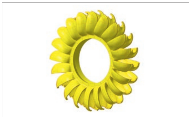
3D de la roue monobloc de la turbine de Montsapay (France) ( Q = 0.350 \text{ m}^3/\text{s} , H_n = 260 \text{ m} , D_{ext} = 1026 \text{ mm} , 750 \text{ t/min} , P_m = 791 \text{ kW} )
